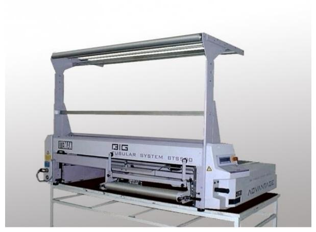
The ADVANTAGE TS is a robust machine specially designed to spread tubular fabrics of different width.
