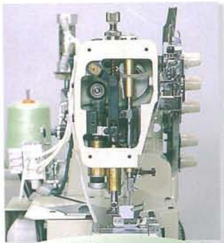
Easily Switchable Needle Bar Stroke
